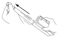
When extending or replacing the antenna, always hold the top of the antenna. Holding the lower part may damage it.
